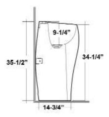
Dimensions of fixture are nominal and may vary within the range of tolerances established by ASME Standard A112.19.2-13. Dimensions and specifications subject to change without notice.
